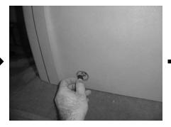
**STEP 2:** Using an 8mm socket, remove the pair of bolts that are located on both sides of the enclosure, towards the rear.
